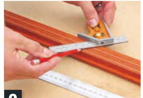
9 Mark the first side to exact length and position against the mitre saw fence. Cramp a stop to the fence and cut two matching pieces
